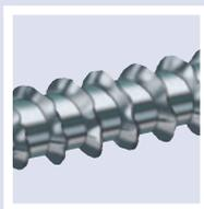
The QZ Combi has flutes at the beginning of the thread, that limit sideways friction in the material. Also every screw has a Hostafalon TF 5032 wax. The resistance when screwing in will be substantially reduced.
