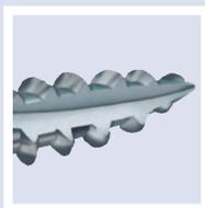
The QZ Combi has a special cutter point that mills out the material when screwing in. That will limit sideways friction in the material and the risk of splitting will be minimalised.
